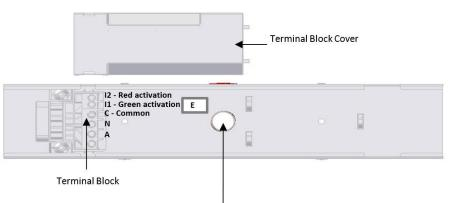
Cable Entry Point – Inside of bracket for ceiling mount, 20mm diameter, located in centre of bracket. Bracket shown with the terminal lock cover removed.
